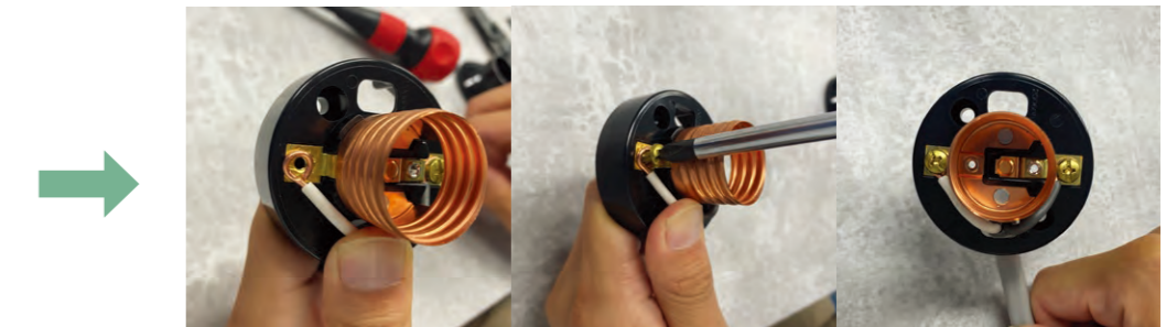
All that's left to do is to align the ring with the screw hole, then screw down the wire with a screw, and you're done!
