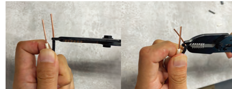
Grip the base of the wire with the stripper and bend it into an L-shape from the base.
