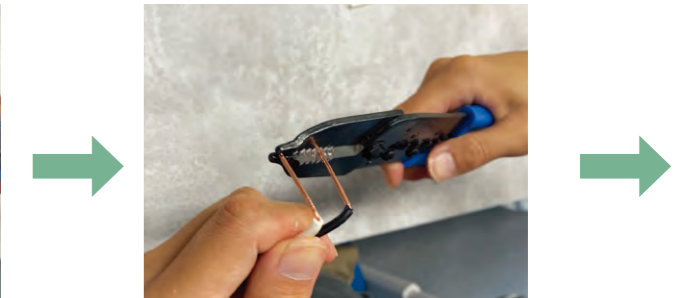
Once the wire is bent into an L-shape, grab its tip and turn your wrist.
