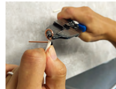
This allows you to bend the wire into a ring shape as shown in the figure.
